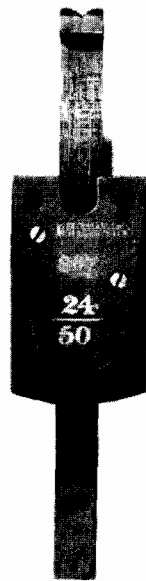
Figure 238. Brass Tangent Scale for Old Brass Guns. (The Royal Artillery Institution, Woolwich, U.K., The Rotunda, XXIV/50.)
