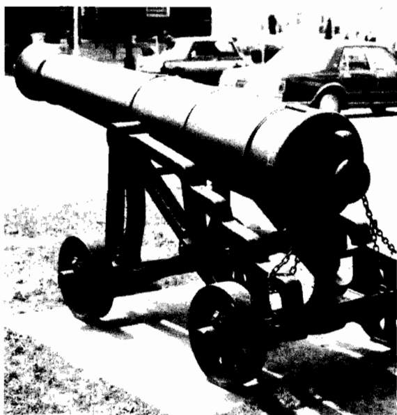
Figure 135. Iron Garrison Carriage for a 24-pounder Gun, weight: 21 hundred-weight 18 pounds. (Near Town Hall, St. Andrew's, New Brunswick.)
