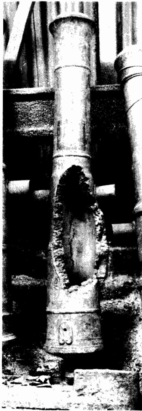
Figure 15. Brass 6-pounder, cast by Richard Gilpin in 1756, weight: 4 hundredweight 2 quarters 22 pounds, length: 4 feet 6 inches. Burst at St. Lucia in 1783. (The Royal Artillery Institution, Woolwich, U.K., The Rotunda, II/48.)
